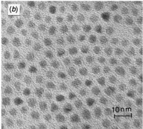
Fig. 3 TEM images of thiol-derivatised Pt (a) and Ag (b) nanoparticles
