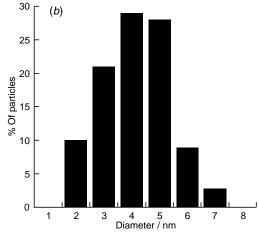
Fig. 2 (a) TEM image of the thiol-derivatised Au nanoparticles forming a superstructure. (b) Histogram showing the size distribution.
