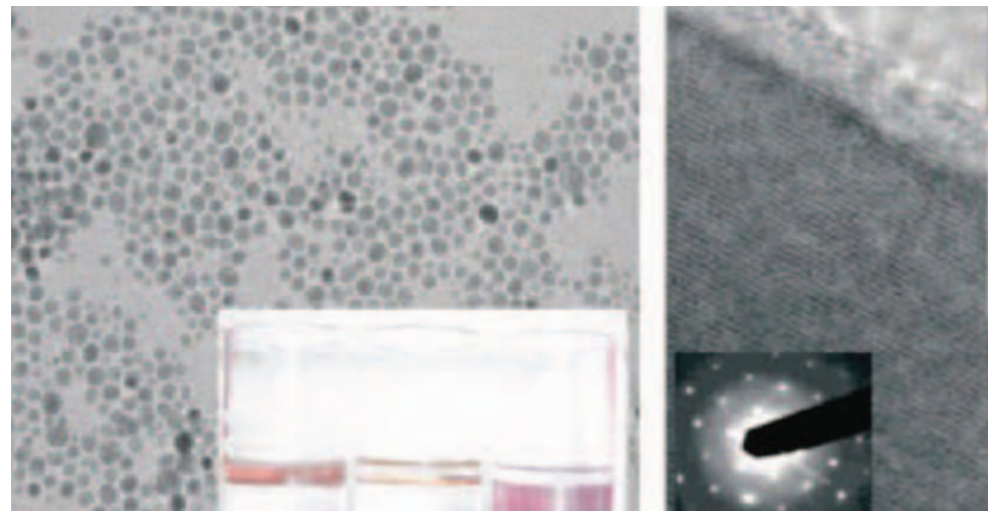
Fig. : Organic-water interface for large scale syntheses of nanocrystals and single crystalline films
