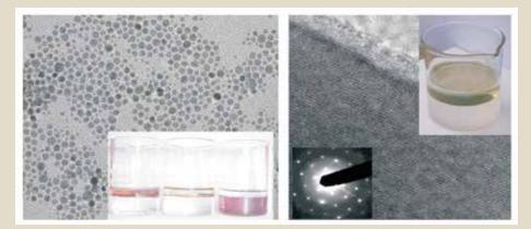
Fig.: Organic-water interface for large scale syntheses of nanocrystals and single crystalline films
