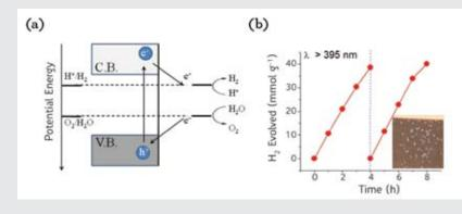
Fig.: (a) Schematic representation and (b) Hydrogen evolution with time
