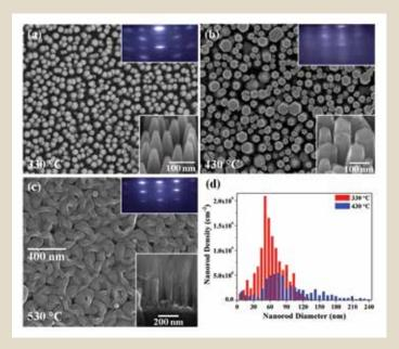
Fig.: Kinetically controlled morphology dependence of InGaN films with different In incorporation
