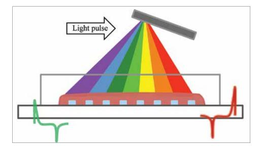
Fig.: Figure depicts a system for focusing various wavelengths of the visible spectrum across a multi-electrode array in accordance with an illustrative embodiment.
