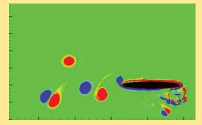
Fig.: Vorticity contours computed close to an elliptical cylinder flapping at Re = 1000
