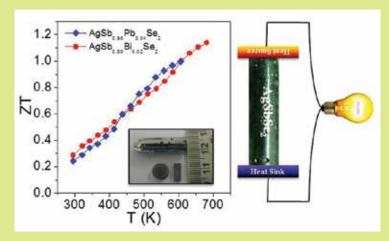
Fig.: High performance thermoelectrics (TE) based on AgSbSe2. Schematic (right) shows TE power generation.
