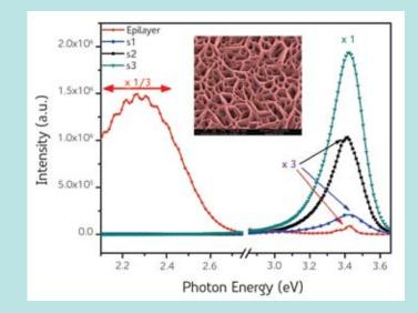
Fig.: Photoluminscence spectra of GaN thin films with different nano-morphologies, showing defect free and enhanced emission in the nanowall-network form.
