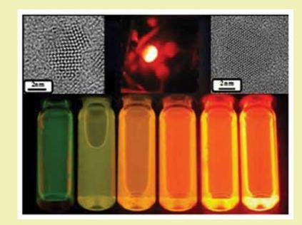
Fig.: Samples under UV-light illumination, TEM images and the LED emission from the same
