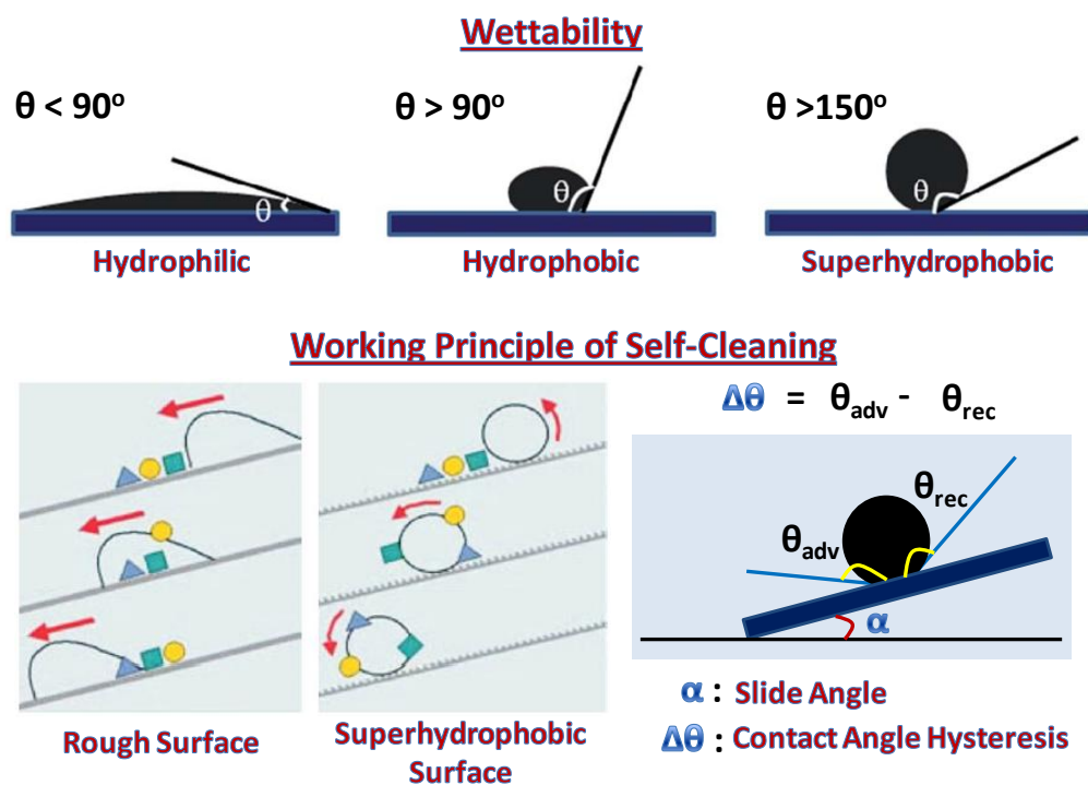
Figure 2. Schematic representation of contact angles for hydrophilic, hydrophobic and superhydrophobic surfaces, and the working principle of self-cleaning. Adapted with permission of RSC from reference 18 and Springer Science and Business Media from reference 19.
