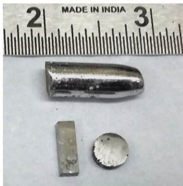
Figure 2.1 Photograph of the as-synthesized ingot. Bar- and coin-shaped samples are used for electrical and thermal transport measurements, respectively.
