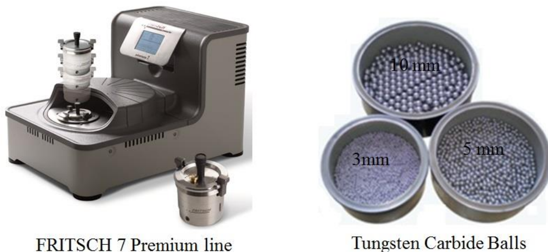
Figure 1.3. Synthesis of intermetallic compounds from micro to nano size by using mechanical milling
