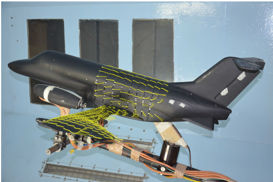
Figure 6.34: Flow visualization for SARAS-O at 14^\circ
