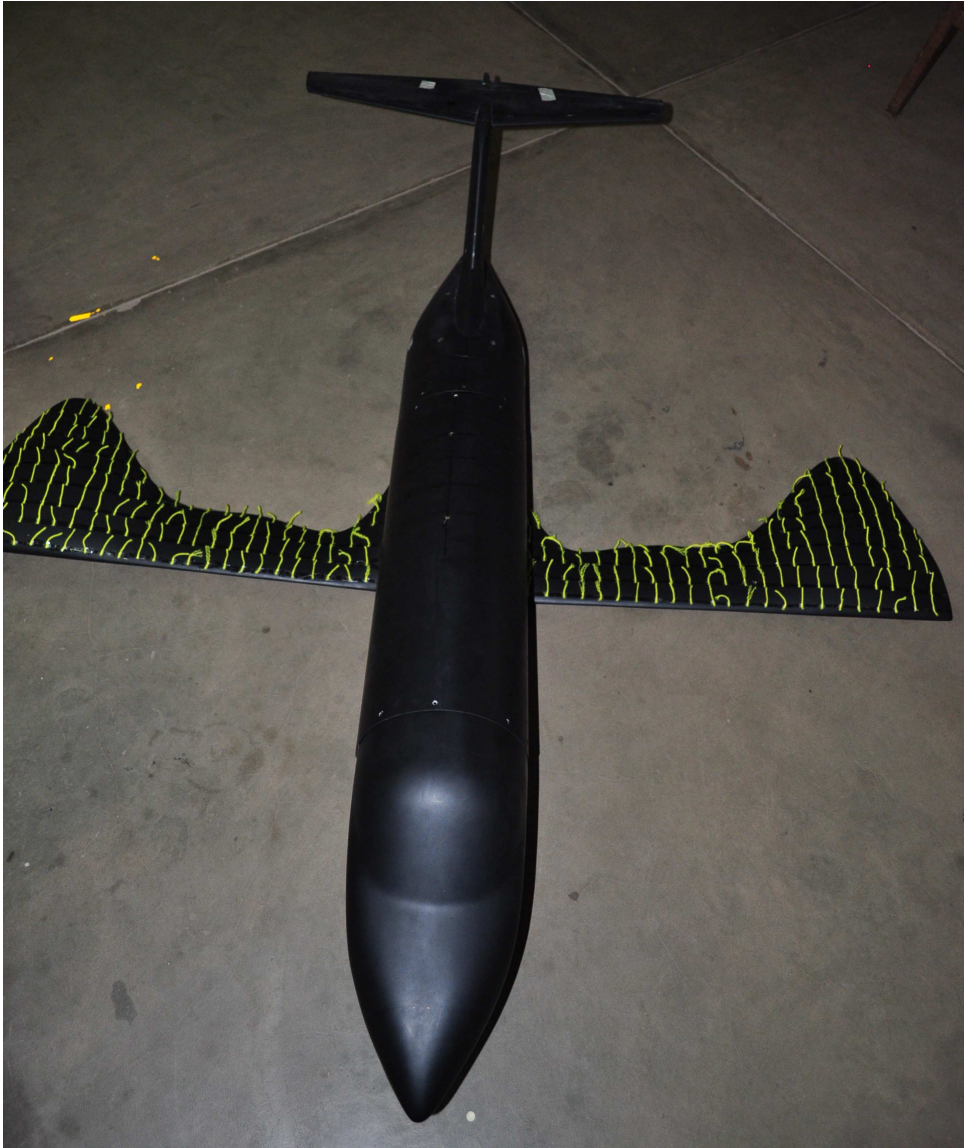
Figure 6.6: Optimal configuration - Saras-o used for wind tunnel testing
