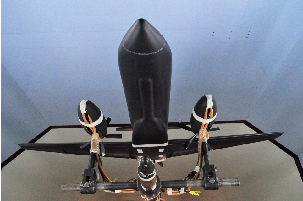
Figure 6.7: Saras wing, as seen from front and below, mounted to the fuselage
