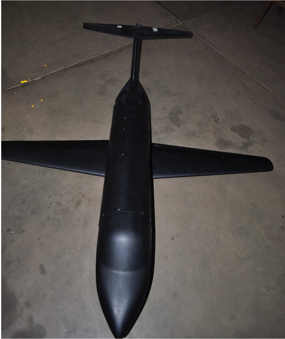
Figure 6.5: Control configuration - Saras-c used for wind tunnel testing
