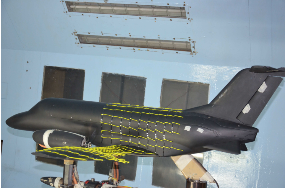
Figure 6.25: Flow visualization for SARAS-O at 0^\circ
