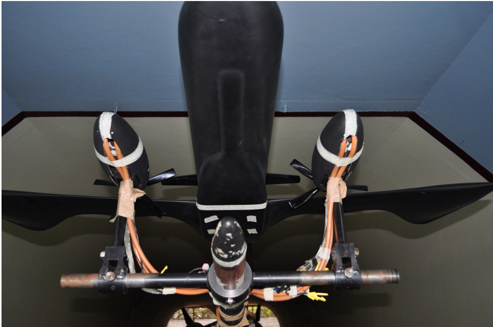
Figure 6.8: Optimal wing, as seen from front and below, mounted to the fuselage
