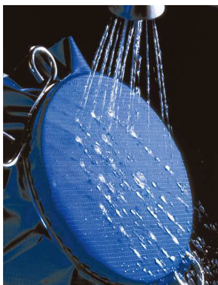
(c) Dirt is removed on smart textiles without wetting, Picture source: http://www.geoffanderson.com/kat16-Fabrics/side301-Sympatex%C2%AE-technology.html
