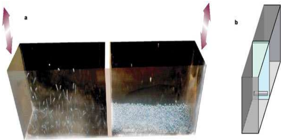
Figure 1.3: (a) Snapshot of spontaneous separation between gas-like and solid-like states of steel beads (diameter 2 mm) from an experiment in which an acrylic container is vibrated sinusoidally at 10 Hz and a maximum acceleration of 1.3g. Initially the beads are distributed uniformly across the container, but owing to collisional inelasticity they migrate to whichever side randomly acquires a slight excess of beads. (b) Schematic of container which is divided into two chambers by a barrier containing a window 6 mm high, beginning 6 mm from the bottom of the container. These figures are taken from Ref. [86].
