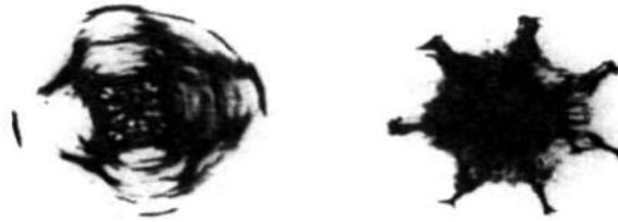
FIGURE 2. Optical intensity patterns for the (4, 3) and (7, 2) modes, respectively. The first index gives the number of angular maxima.
