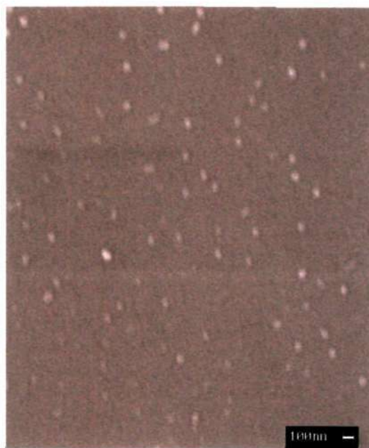
Figure 2.2: SEM picture of 2% wt. ratio of TiO 2 with respect to MEH-PPV.
