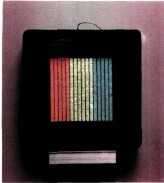
Figure 1.9: Emitting image of a fully sealed 4.5" SWNT-FE display (developed by Samsung Corp. [64]).
