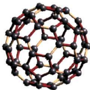
Fig. 1.9 \text{C}_{60} molecule is polygon with 60 vertices and 32 faces, 12 of which are pentagonal and 20 hexagonal, having a truncated icosahedron structure [36].
