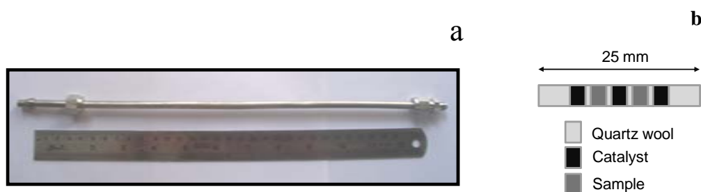
Figure 11: a) Digital photography image showing the stainless steel reactor tube b) Cartoon depicting the packing of the catalyst and sample at the centre of the reactor tube.
