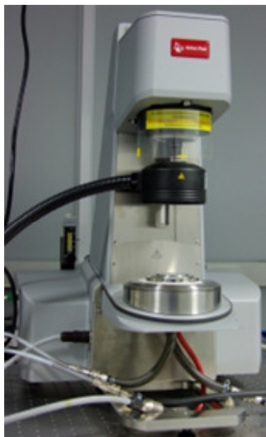
Figure 1.2.3 Rheometer (MCR 301-WESP) used for the study of gel samples.
