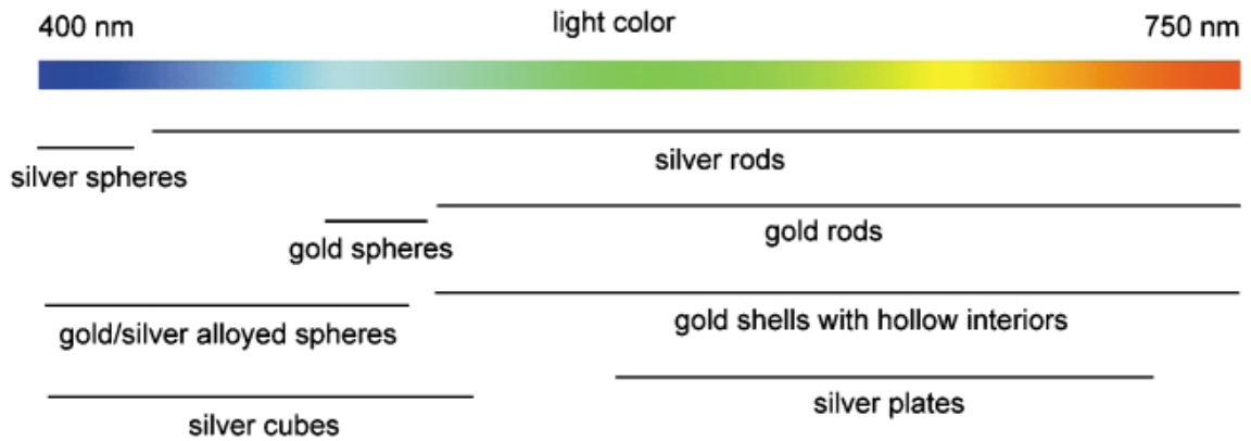
Figure 3.1: SPR band of different nanoparticles [11].
