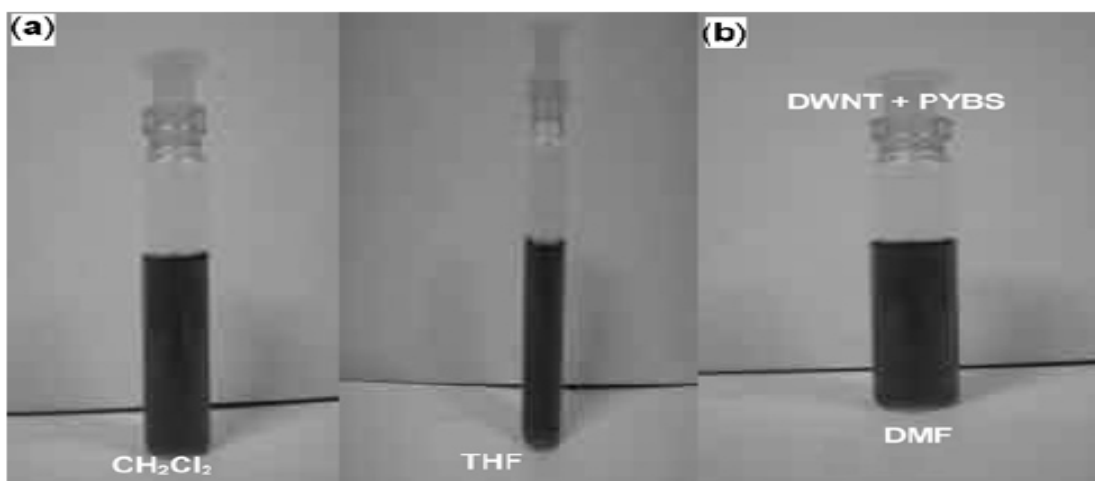
Fig. 4.11 Photographs of vials containing the dispersions of DWNTs in various solvents: (a) amide-functionalized DWNTs, (b) PYBS functionalized DWNTs.
