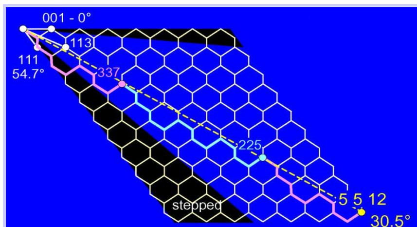
**Fig. 2.7:** Bulk truncated Si viewed from (100). The composition of Si(5 5 12) surface is indicated.
