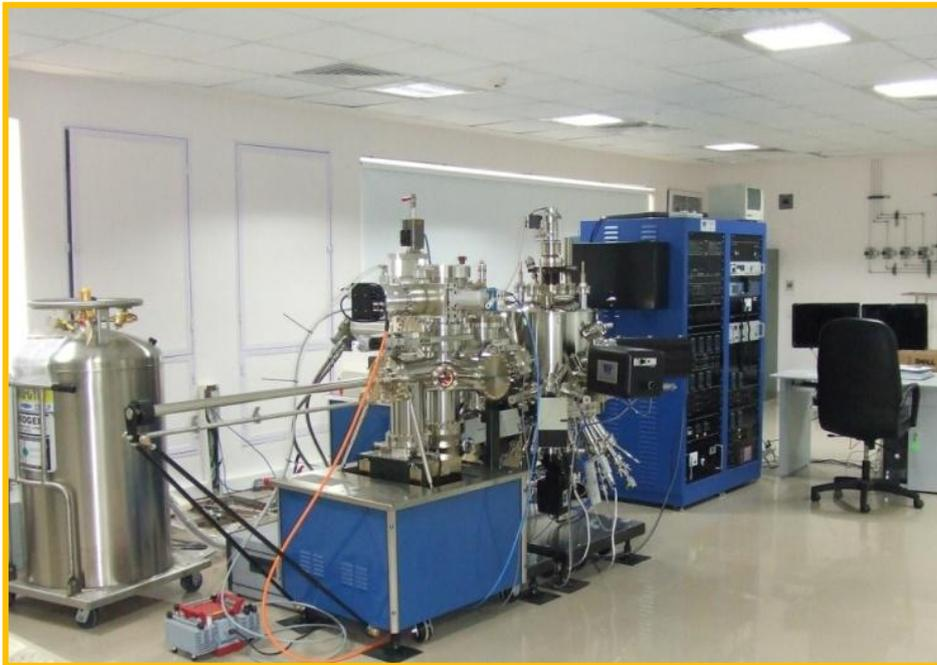
**Fig. 3.13:** SVTA MBE system used in the present study for the growth of InN and GaN films
