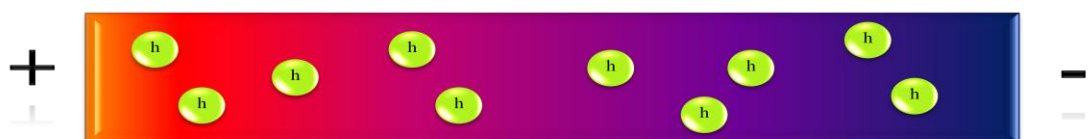
Fig.3.26: flow of charge carrier in a p-type material under thermal gradient
