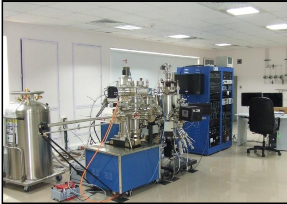
Fig. 3.2: SVTA MBE system used for growing GaN nanowall network.
