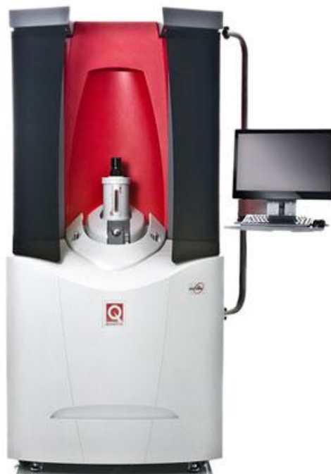
Fig 3.10: SQUID used for the magnetic studies in the present work, Quantum Design, Inc.
