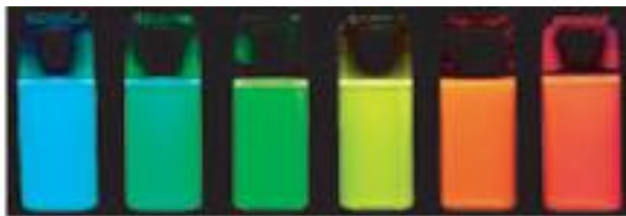
Figure-4: Fluorescence of CdSe–ZnS core–shell nanoparticles with diameter of 2.7 nm (blue) up to 5 nm (red), giving evidence of the scaling of the semiconductor band gap with particle size (Ref. 26- reprinted with permission).
