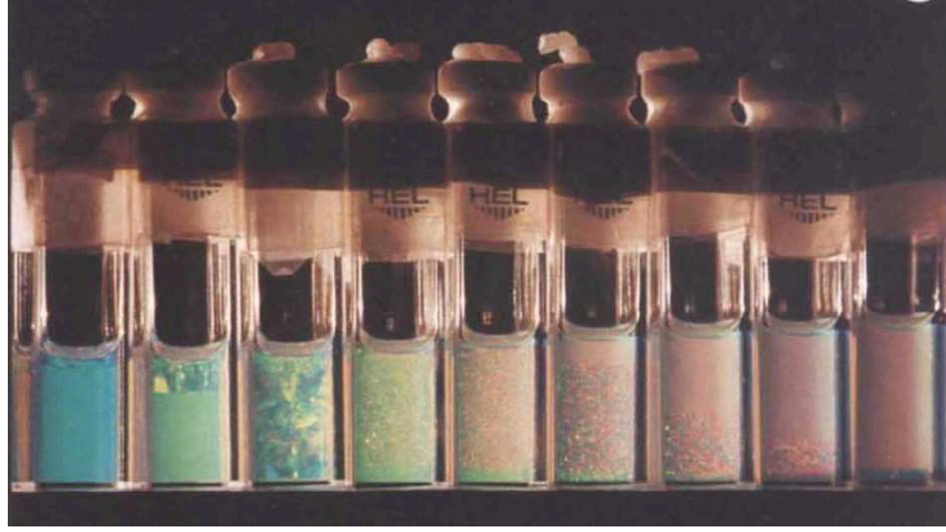
Figure 1.7: Nearly hard spheres colloidal suspension, 4 days after tumbling. States of the suspensions from left, first - fluid; next three - liquid-crystal coexistence; next two - homogeneous crystal; 7 th - heterogeneous crystal; last two - glass. Bragg scattering can be observed in crystalline samples. The last sample did not crystallize even after several months. Adopted from. 47
