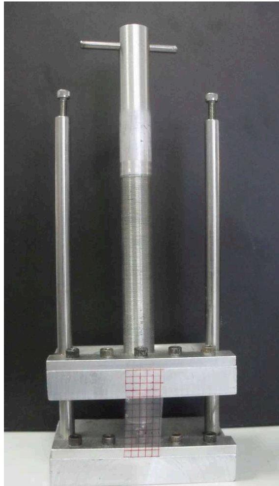
Figure 2.2: Stretching apparatus built in our lab. The film is clamped in between two steel blocks as shown and stretching is done manually.
