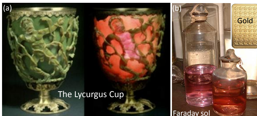
Figure I.2 (a) The apparent dichroism of Lycurgus cup towards the direction of light illumination and (b) gold sol prepared by Michale Faraday. Inset, bulk gold is in yellow color [reproduced from ref. 4, 5].
