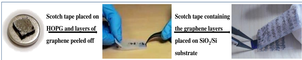
Figure II.1 Schematic showing the steps followed in the scotch tape technique to get few layers of graphene.
