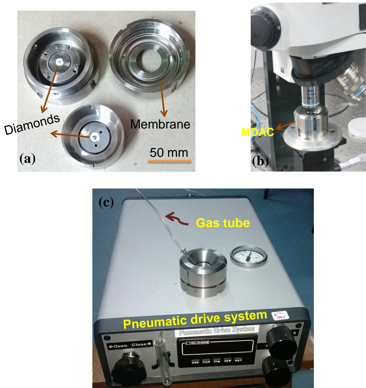
Figure 2.6: Photograph of the a) MDAC b) MDAC under Raman microscope c) MDAC connected to pneumatic drive system (PDS).
