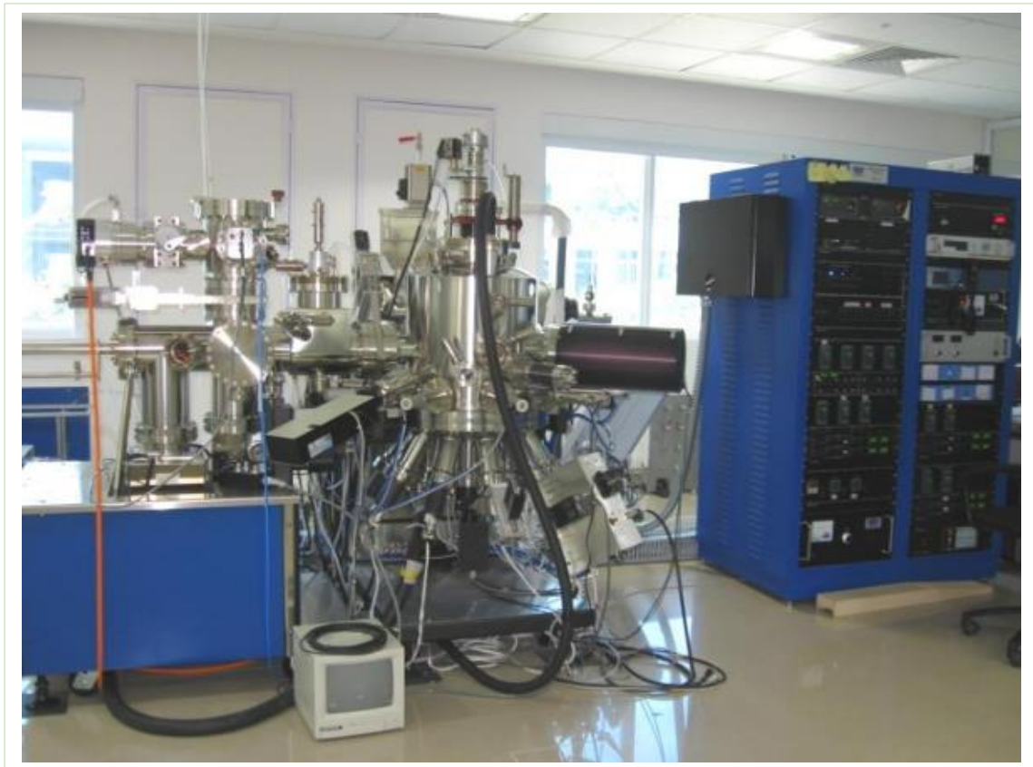
Fig A.2.2: SVTA MBE System used in the present study for the growth of GaN films.
