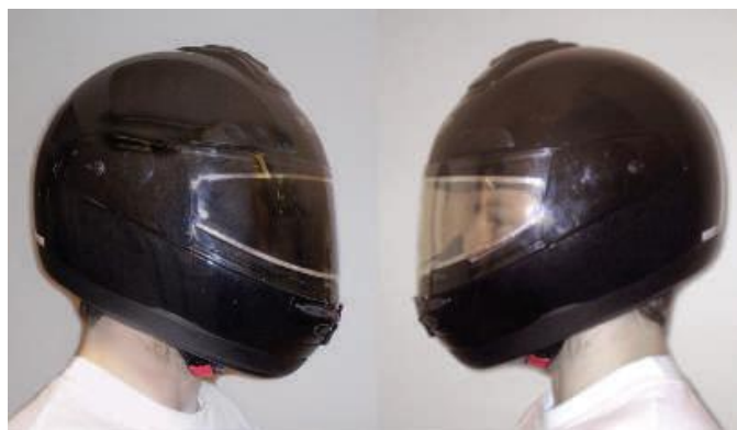
Figure 2: Motorcycle helmet with visor based on electrochromic foil, in dark and transparent state. The clear-state transmittance was deliberately set to 50%, although new EC materials can give more than 80% transmittance. Adapted with permission from reference 29. Copyright 2006, Nature Publishing Group.
