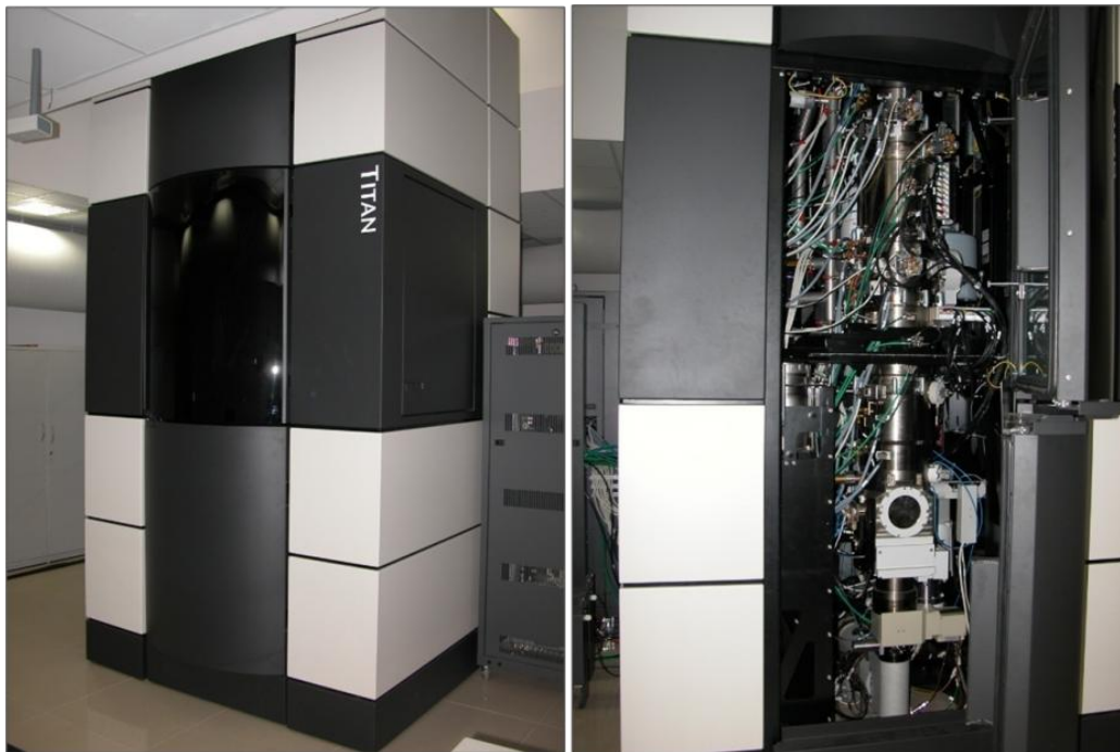
Figure 2.2. FEI TITAN 3 ™ 80-300 kV at International Centre for Materials Science (ICMS), Jawaharlal Nehru Centre for Advanced Scientific Research (JNCASR), Bangalore. It has double Cs corrector technology with both image and probe corrector systems.
