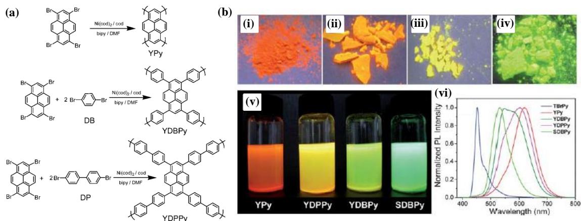
Figure 20. (a) Synthetic routes to luminescent CMPs showing notional network structures. The actual structures of these statistical copolymers will be more complex than represented. (b) Photographs of the polymers under irradiation with UV light ( \lambda_{\text{ex}}=365 nm) in the solid state, (i) YPy, (ii) YDPPy, (iii) YDBPy, and (iv) SDBPy; (v) Photographs of suspensions of the polymers in THF (10 mg/10 mL); (vi) Photoluminescent spectra of the monomer TBrPy and the resulting polymers measured in solid state powder ( \lambda_{\text{ex}} = 360 nm). These figures have been reproduced with permission from reference no 40d.
