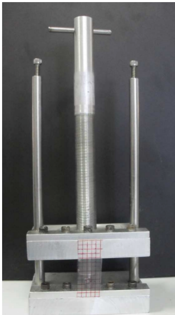
Figure 2.10 The film stretching apparatus, developed in-house. The film is clamped in between two aluminium blocks as shown and stretching is done manually.
