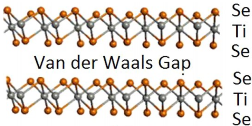
Figure 3.3. Schematic of the layered structure of \text{TiSe}_2 adapted with permission from Nano Lett. 12,11,5941-5945 . Copyright(2012) American Chemical Society.
