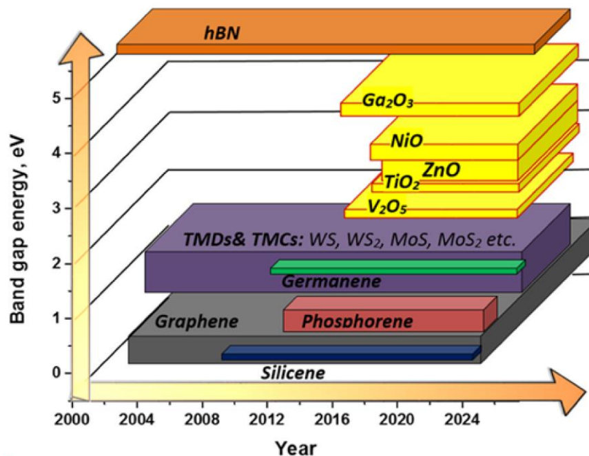
Figure 15. Evolution of the family of 2D materials as a function of time and their respective band gap values. The yellow slabs indicate the expected 2D metal oxides contribution. Reproduced with permission from ref. [154]
