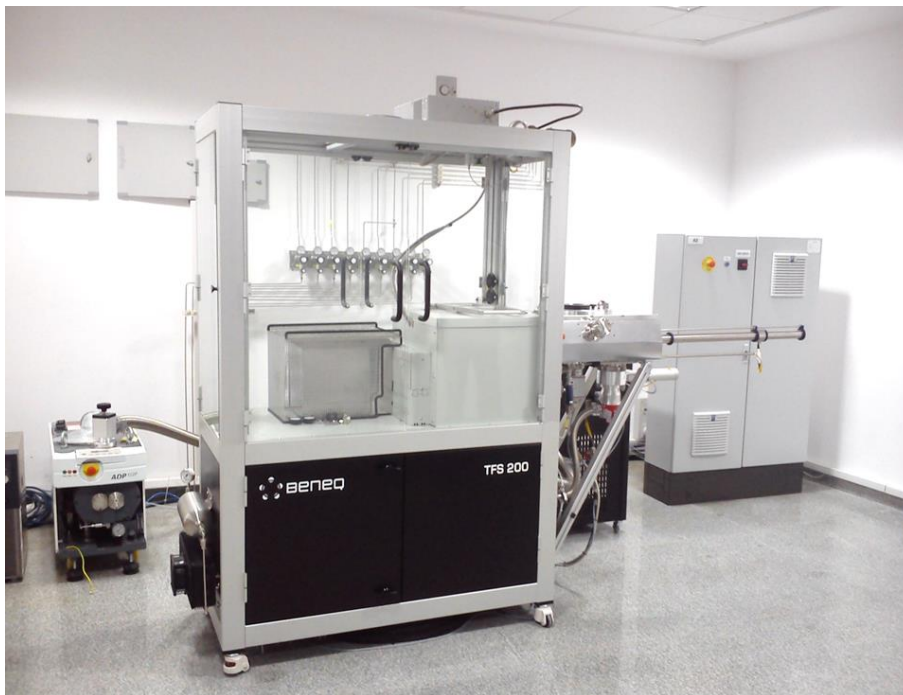
Figure 4. Photograph of Beneq TFS-200 ALD system installed at JNCASR, Bengalore (India).
