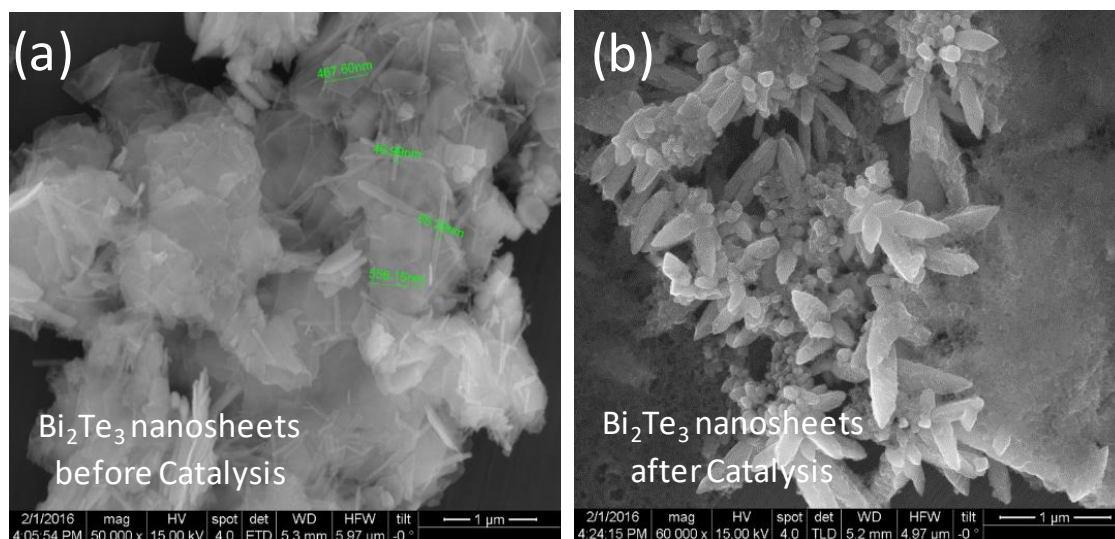
Figure 24. SEM images of \text{Bi}_2\text{Te}_3 before and after HER studies. We observe morphology changes after HER.
