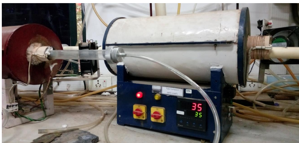
Figure 2.14 Laboratory fabricated furnaces usable up to 1150 °C according to the temperature profile given in the controller.
