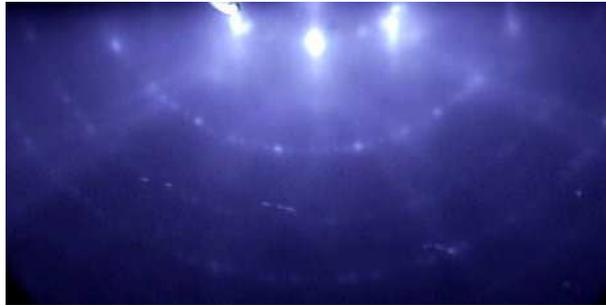
Figure 7.1: RHEED pattern of  $7 \times 7$  reconstructed surface of Si(111).
