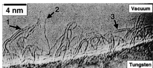
Fig. 36 HREM image of single-walled BN nanotubes adhering on a W substrate. (Reproduced with permission from ref. 110).
