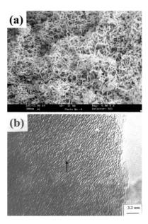
**Fig. 2** (a) SEM image of as-synthesized carbon fibres; (b) HREM image of carbon fibres showing the stacking of graphitic planes. The arrow denotes the direction of growth of the fibre.
