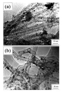
Fig. 6 Low magnification TEM images of (a) Pt-decorated MWNTs, and (b) Pd-decorated MWNTs.
