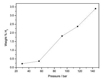
Fig. 4 Hydrogen storage in aligned MWNTs (acid-treated), sample IX,
