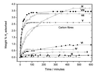
Fig. 3 Amount of hydrogen adsorbed in wt% as a function of time for the various carbon nanostructures. The broken curve represents the blank data obtained in the absence of a carbon sample.
