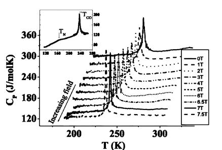
FIG. 2. Waterfall plot of specific heat as a function of temperature at various magnetic fields. Note that the data are offset for clarity. Inset: Specific heat as a function of temperature for zero field over an extended temperature range. Note the  $T_{CO}$  at  $\approx$ 235 K and  $T_N$  at  $\approx$ 165 K.
