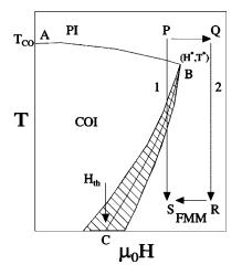
FIG. 1. A cartoon of the  $T-\mu_0 H$  plane phase diagram seen in most manganites like  $Pr_{1-x}Ca_xMnO_3$  which show the onset of CO transition from a PI (charge disordered) state. COI is charge-ordered insulator and FMM is ferromagnetic metal.
