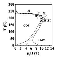
FIG. 6.  $T - \mu_0 H$  plane phase diagram of  $Pr_{0.63}Ca_{0.37}MnO_3$  combining the results of the present investigation and the existing phase diagram (solid line). *M* is metallic phase.
