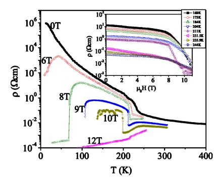
FIG. 5. Resistivity as a function of temperature for a few representative fields. Inset shows resistivity as a function of field at different temperatures.
