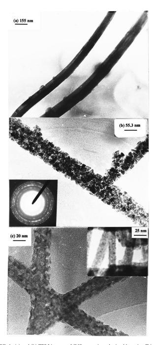
FIG. 1. (a) and (b) TEM images of CdS nanowires obtained by using Triton 100-X as the surfactant. Inset (b) shows the electron diffraction pattern of the CdS nanowires; (c) shows TEM images of CdSe nanowires obtained by using Triton 100-X as the surfactant.
