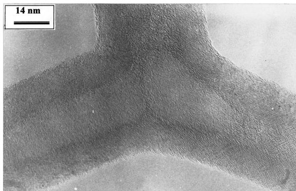
FIG. 3. HREM image of a Y junction showing the fishbone-type stacking of graphene sheets ( d_{(002)} \sim 3.4 \text{ \AA} ).
