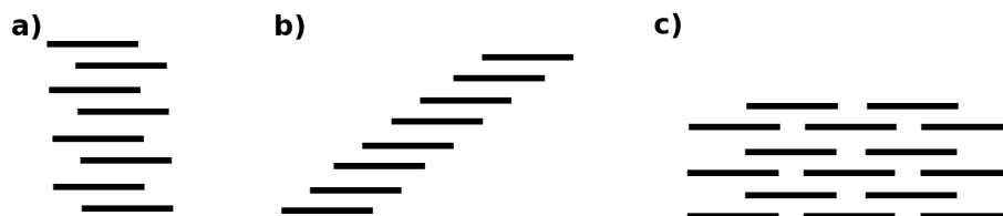
Figure 1.6: Schematic representation of the different arrangements of chromophores in J-aggregates. (a) Ladder-type, (b) Staircase-type and (c) Brickwork type
