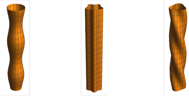
Fig. 1.1 Three possible variations of the perturbations of a liquid column - axisymmetric perturbations (left), Planar perturbations (middle) and three-dimensional perturbations (right).
