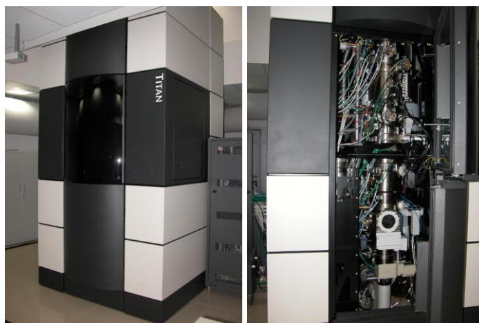
Figure 1.04. FEI TITAN 80-300 kV transmission electron microscope with a double aberration corrector.
