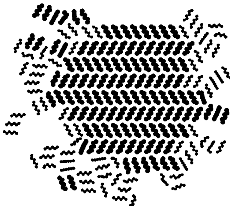
Figure 5.2: Top view of the time averaged configuration of the first adsorbed layer of n -hexane multilayer on graphite. Molecules in black have at least one intermolecular distance that is less than 5.0\text{\AA} . Hydrogen atoms are not shown for clarity.
