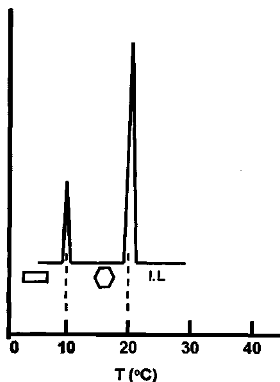
Figure 1.9: DSC trace of an odd-alkane, heptadecane (C 17 ) is shown. The peak at 10°C represents the transition from a tightly packed orthorhombic crystal to a pseudo-hexagonally packed crystal. The peak at 21°C signifies the melting transition. Both transitions are sharp with enthalpies of 2.5 and 9.2 kcal/mol, respectively [Adopted from Ref. [1]].
