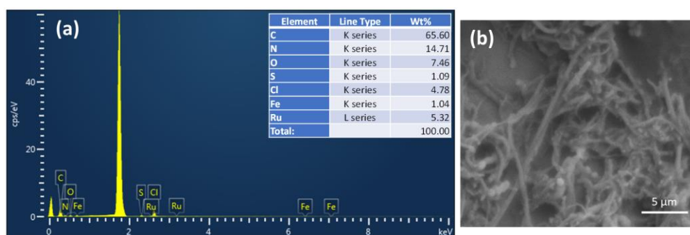
Figure 9. (a) FESEM and (b) EDAX analyses for Fe 2 @CPG after the fourth catalytic cycle.
