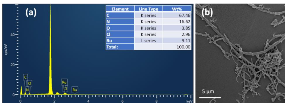
Figure 3. (a) EDAX analysis and (b) FESEM image of Ru-TPY-POR CPG after performing photocatalytic water reduction experiment (with TEA) up to 4 th cycle under visible light irradiation.
