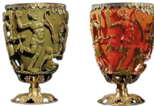
Figure 1.4 Ancient Roman Lycurgus cup. It appears green in reflected light while red in transmitted light. These glasses are mixed with gold nanoparticles (typically 10–100 nm in size). 16
