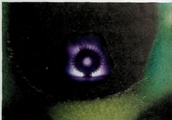
Fig. 2.7 Application of plasma in industry. The plasma is used for surface hardening of a gear wheel kept in the discharge chamber by the process of Nitriding (courtesy: P.K. Kaw, Institute of Plasma Research, Gandhinagar, Gujarat).
