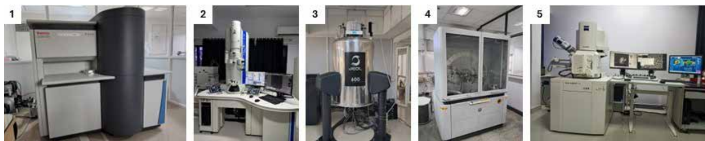
Image: Photographs of some of the high-end equipment that SRF offers access to. (1) X-ray photoelectron spectroscope (ThermoFisher); (2) Transmission electron microscope JEOL JEM 2100 plus; (3) Nuclear magnetic resonance JEOL 600 MHz; (4) Powder X-ray Diffractometer; (5) Field Emission Scanning Electron Microscope (Zeiss GeminiSEM500).
