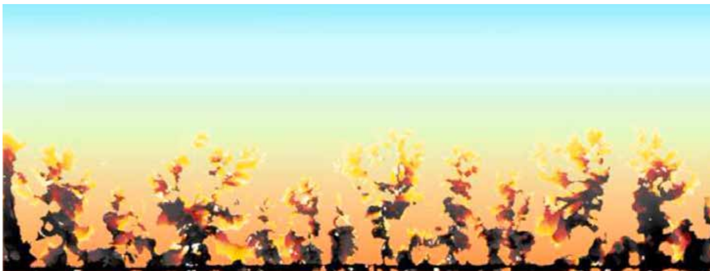
Dendrite formation during electrodeposition of copper from copper sulphate.
