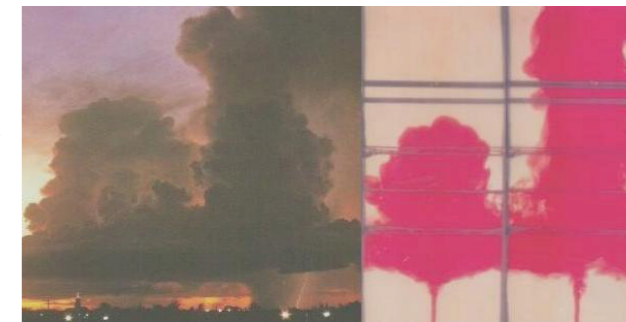
Figure 2: Real clouds (left) and fake clouds in the laboratory (right). The latter are generated by dumping ohmic heat into a plume of electrically conducting fluid in a water tank of size 600 mm × 600 mm.
