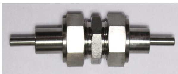
Figure 2. A homemade stainless steel cell is used for battery assembly.
