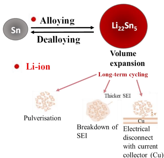
Figure 1. Illustration depicting the lithium-tin (Li-Sn) alloy formation process and the challenges during prolonged cycling.[17]
