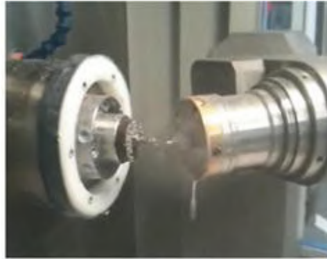
Fig. 1.8 Polishing of micro-mold (Source: Beaucamp et al. [5])
